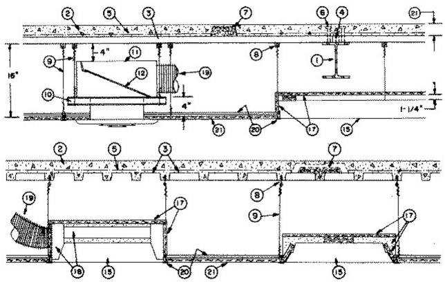
1. **Beam** — W8x15, min size. As an alternate to steel beams, standard steel joists, Type 10J3, 12K1 or LH Series joists of any size may be used as an alternate to steel beams. Joist girders, 20 in. min depth and 13 lb/lin ft min weight may also be used as alternate to steel beams.
