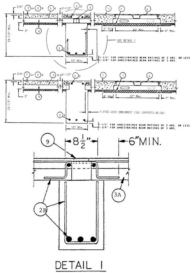
**Supports** — W8x28 or W6x12 min size steel beams, or steel joists, composite or noncomposite. Steel joists shall be welded to end supports. Min area of joist members shall be 1.44 sq in. for top chord angles, 0.87 sq in. for bottom chord members and 0.47 sq in. for web members. Bridging angles required for noncomposite steel joist, min 1-1/4 in. by 1-1/4 in. by 1/8 in.
