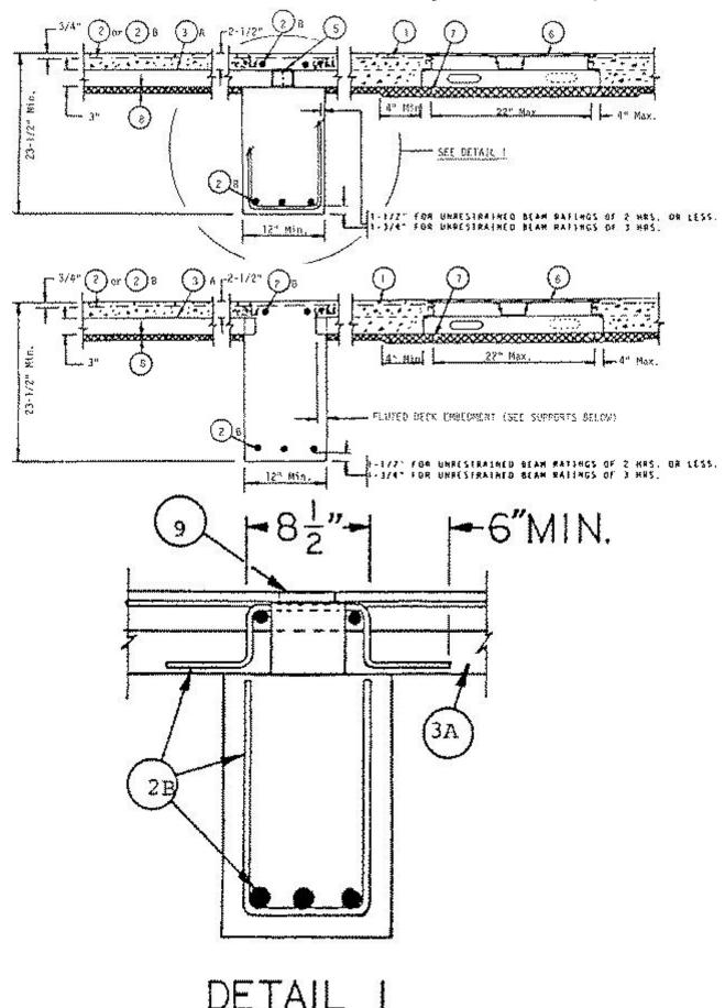
**Supports** — W8x28 or W6x12 min size steel beams, or steel joists, composite or noncomposite. Welded to end supports. Min area of joist members shall be 1.44 sq in. for top chord angles, 0.87 sq in. for bottom chord members and 0.47 sq in. for web members. Bridging angles required for noncomposite steel joist, min 1-1/4 in. by 1-1/4 in. by 1/8 in. thick. Welded to the
